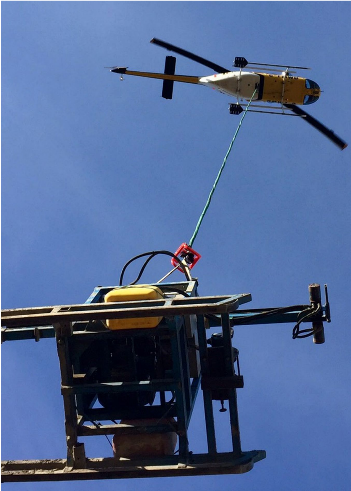
Figure 6: Heli-portable Reverse Circulation (RC) drill rig
