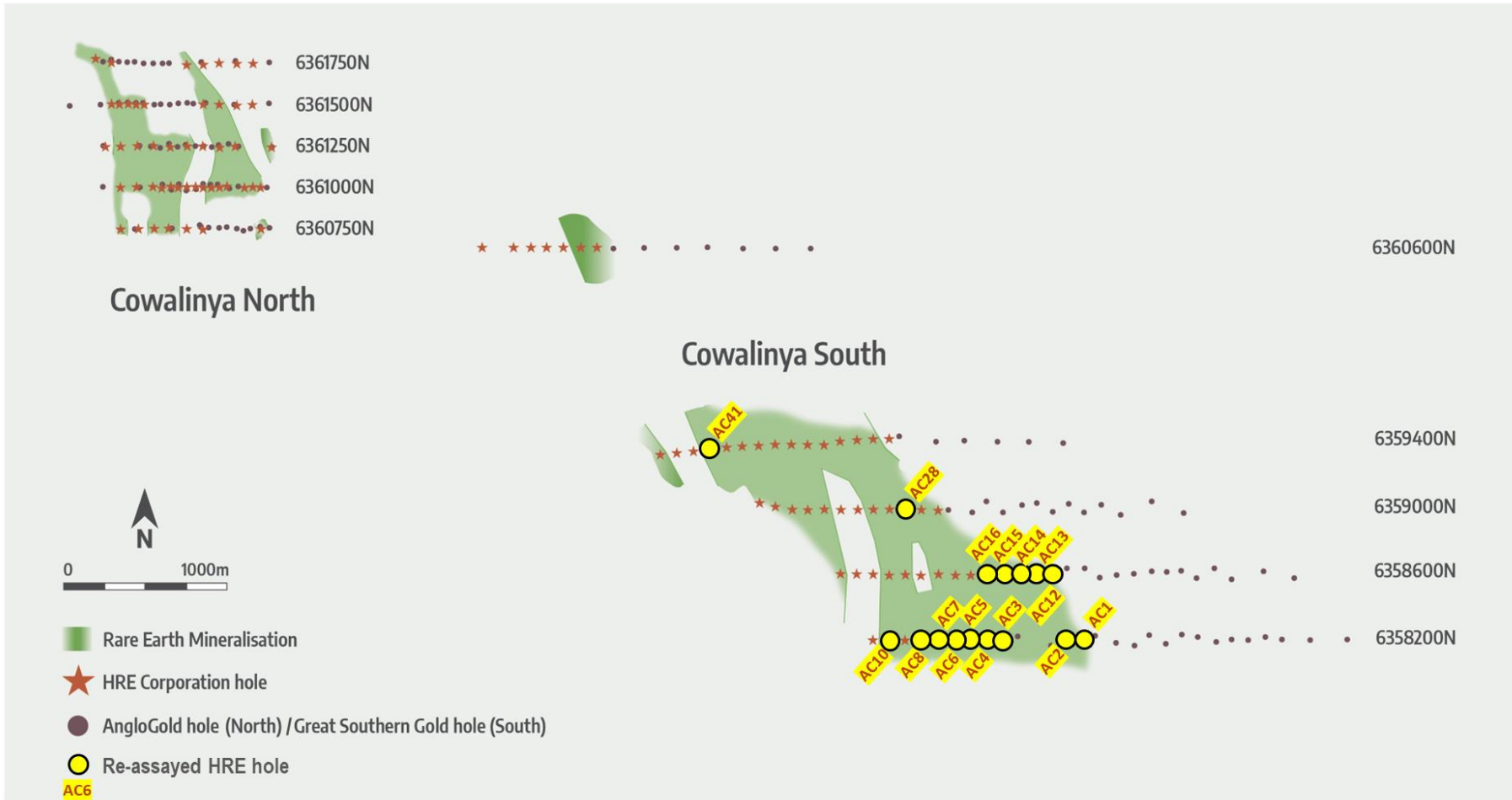
Figure 1: Plan view of Cowalinya deposit air core drilling. Drill holes from which re-assays are reported in Table 1 are shown in yellow.
