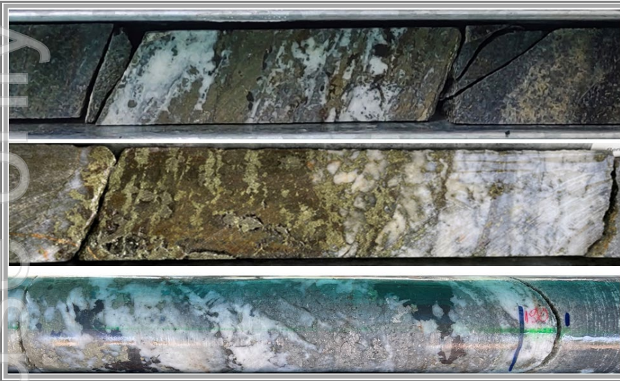
Figure 14 | Mineralised veins in Memot Diamond Core
