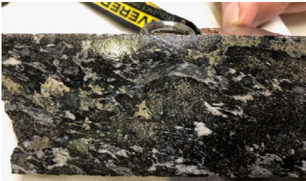
Left: Core from 236m depth within PDD002 showing disseminated and semi-massive sulphide as void infill within strongly altered breccia. Below: Drill core from PDD003 (below, top tray) and PDD004 (below, bottom tray); both showing brecciated zones with hydrothermal alteration.
