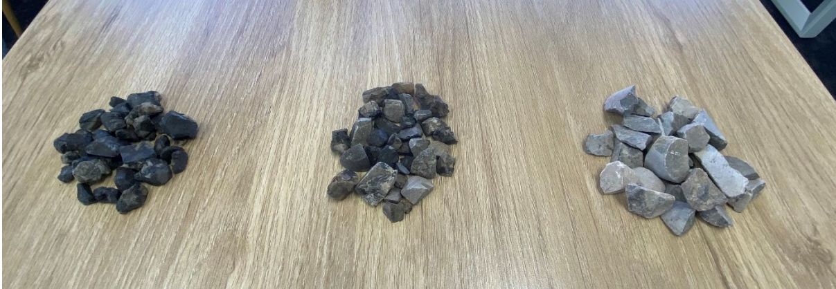
Figure 20: The three products produced from the ore sorting test work. Left to right – Very High Density product (DSO), High Density product, and Low Density product (waste rock)
