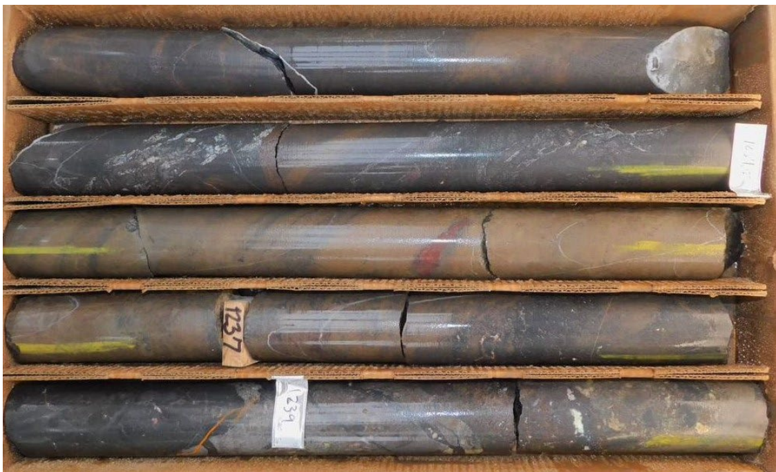
Figure 8: Photo of massive and semi-massive sphalerite (zinc sulphide – brown) and magnetite in drill hole WD22-03. This interval contains 47.59% Zn, 435.88g/t In from 376.26 – 377.02m (1234.5 - 1237ft) downhole.
