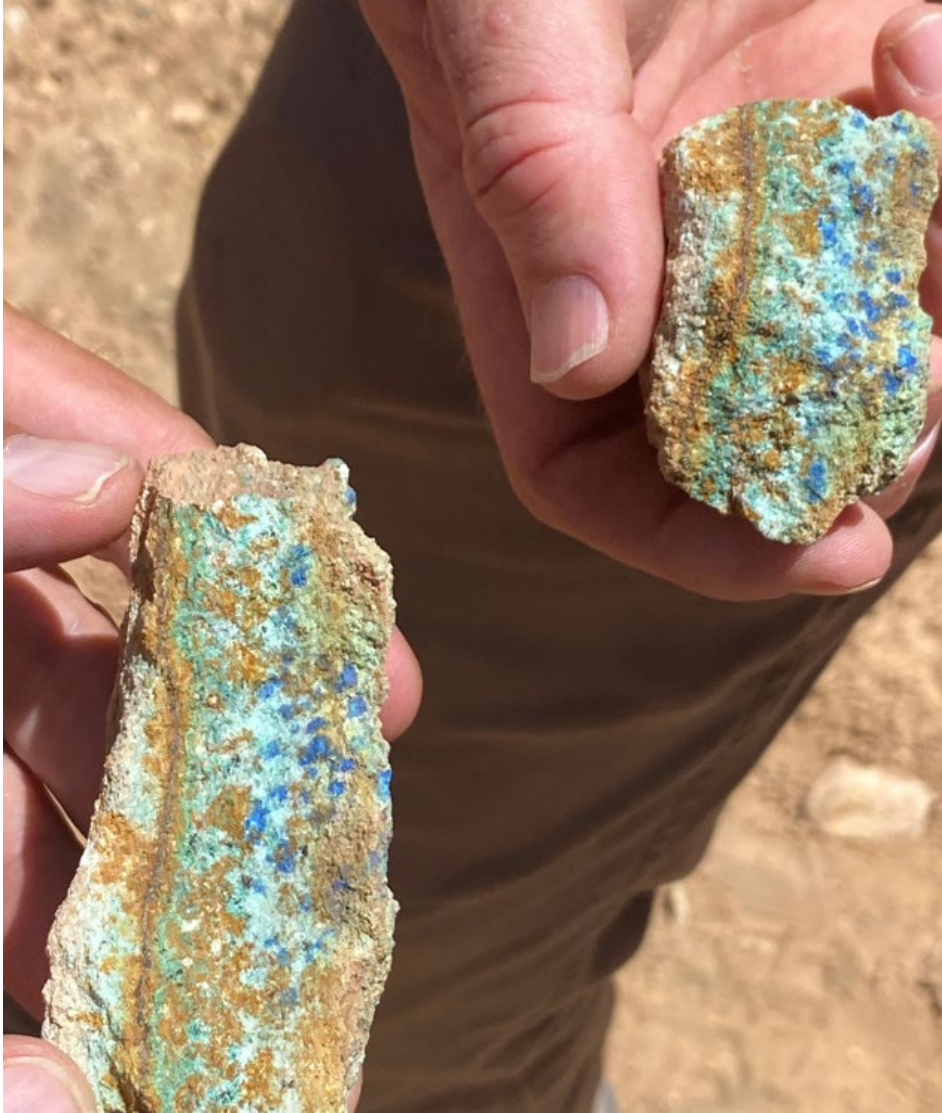
Figure 31: Recent rock sample showing heavily disseminated azurite (blue mineral – derived from oxidised chalcocite) within coarse grained sandstone. This sample is taken from outcropping Dakota Formation within the Copper Warrior Project.
