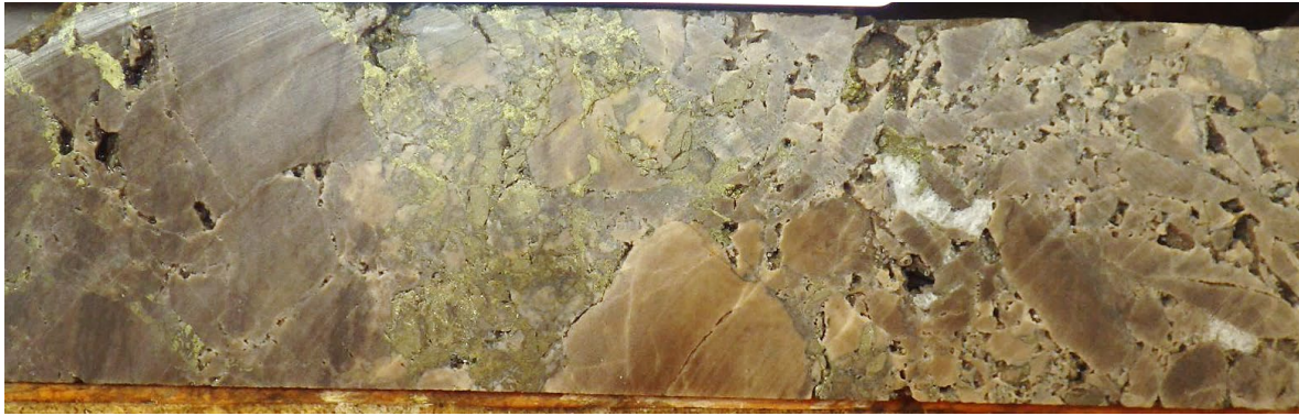
Figure 25: Chalcopyrite (copper sulphide) within ST22-10 drill core from 313m downhole.
