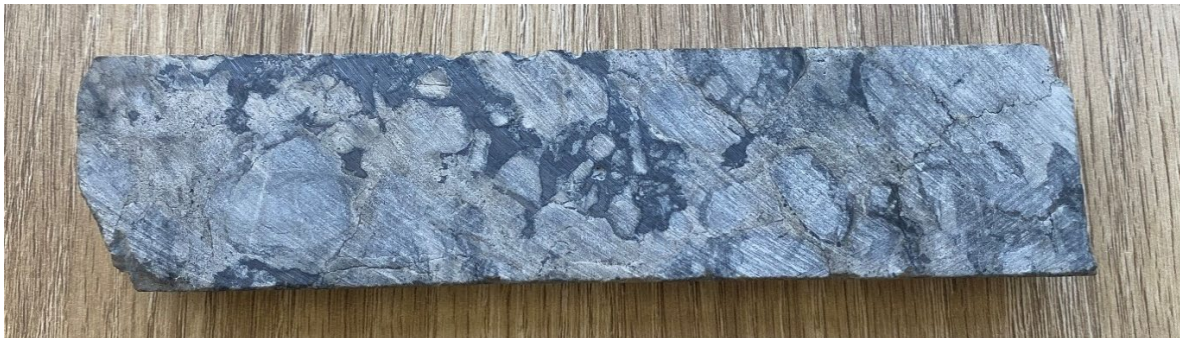
Figure 19: Drill core from STOR1601D from interval 97-101m downhole – average grade 4.16%. The Chalcozite is seen as the dark gunmetal grey material within the lighter grey dolomite host rock.
