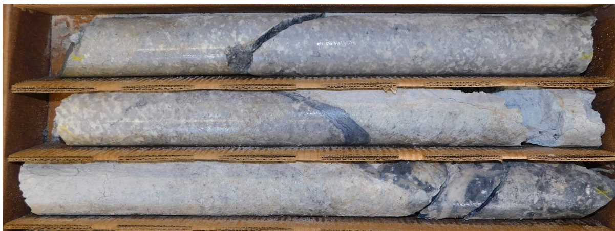
Figure 6: Strong molybdenite veining in drill core from WD22-01 (761 – 763.5m downhole)
