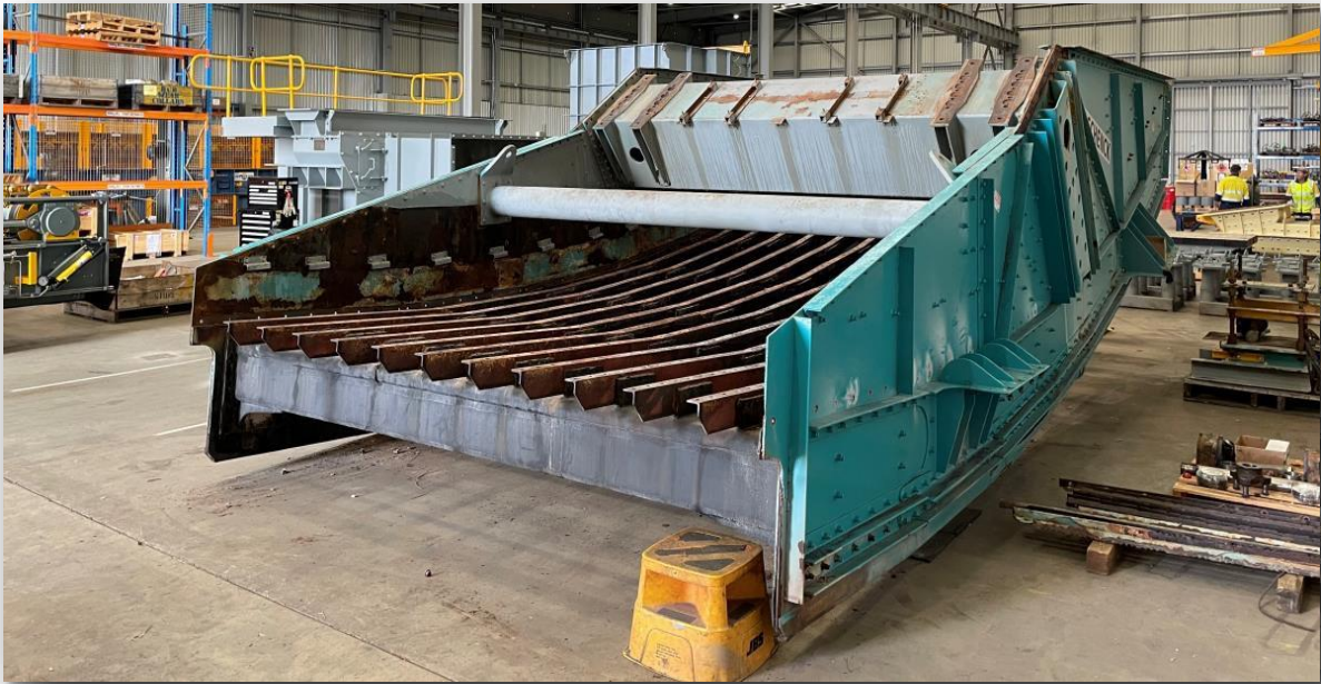
Figure 5: Schenck screen being refurbished at RCR
