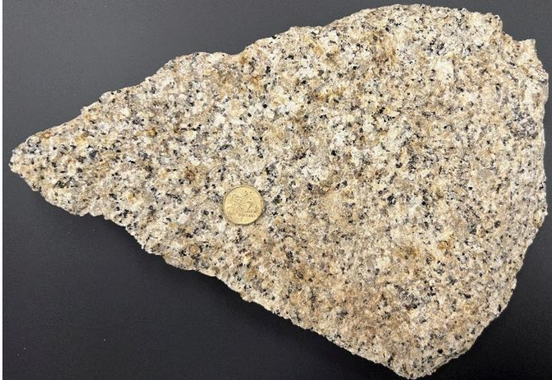
Figure 4. Specimen of oxidised monzogranite (Venus sample 22056540A, TREO of 1407 ppm) with brownish REE mineralisation.
