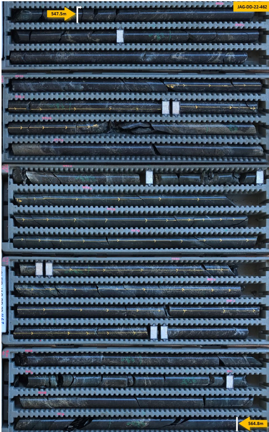
Figure 11 – Core photo from drill hole JAG-DD-22-462 (Onça Preta); 547.5m to 564.8m down-hole: Disseminated, stringer to semi-massive sulphides (metallic bronze/yellow colour) with intense magnetite (black colour) mineralisation hosted in basement gneiss.
