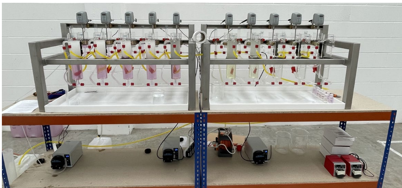
Figure 6: Mixer-settler circuit as part of the magnet recycling pilot plant being commissioned at the new Ionic Technologies facility located at the Titanic Quarter in Belfast, UK. The first 5 stages show the separation of Didymium (NdPr) from Dysprosium (Dy) in the last two stages.
