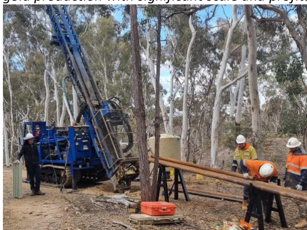
Figure 1 Diamond rig collared on a hole on the Red Hill Gold resource
