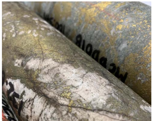
Figure 8: Stringer Zone chalcopyrite mineralization in QMines drill core, hole MCDD018.
