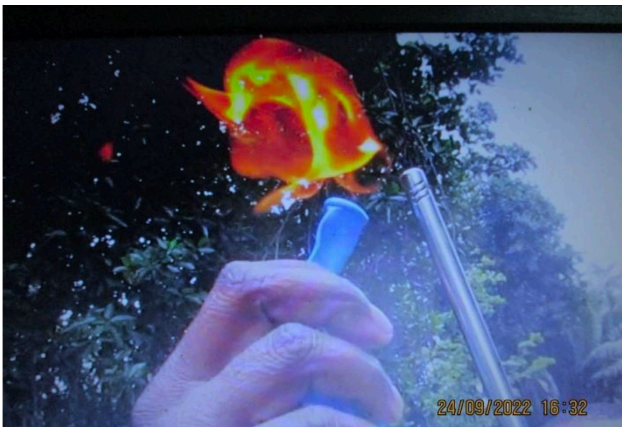
Figure 2. Field-testing of gas bubbling from reservoir rock beneath Alligator Creek
