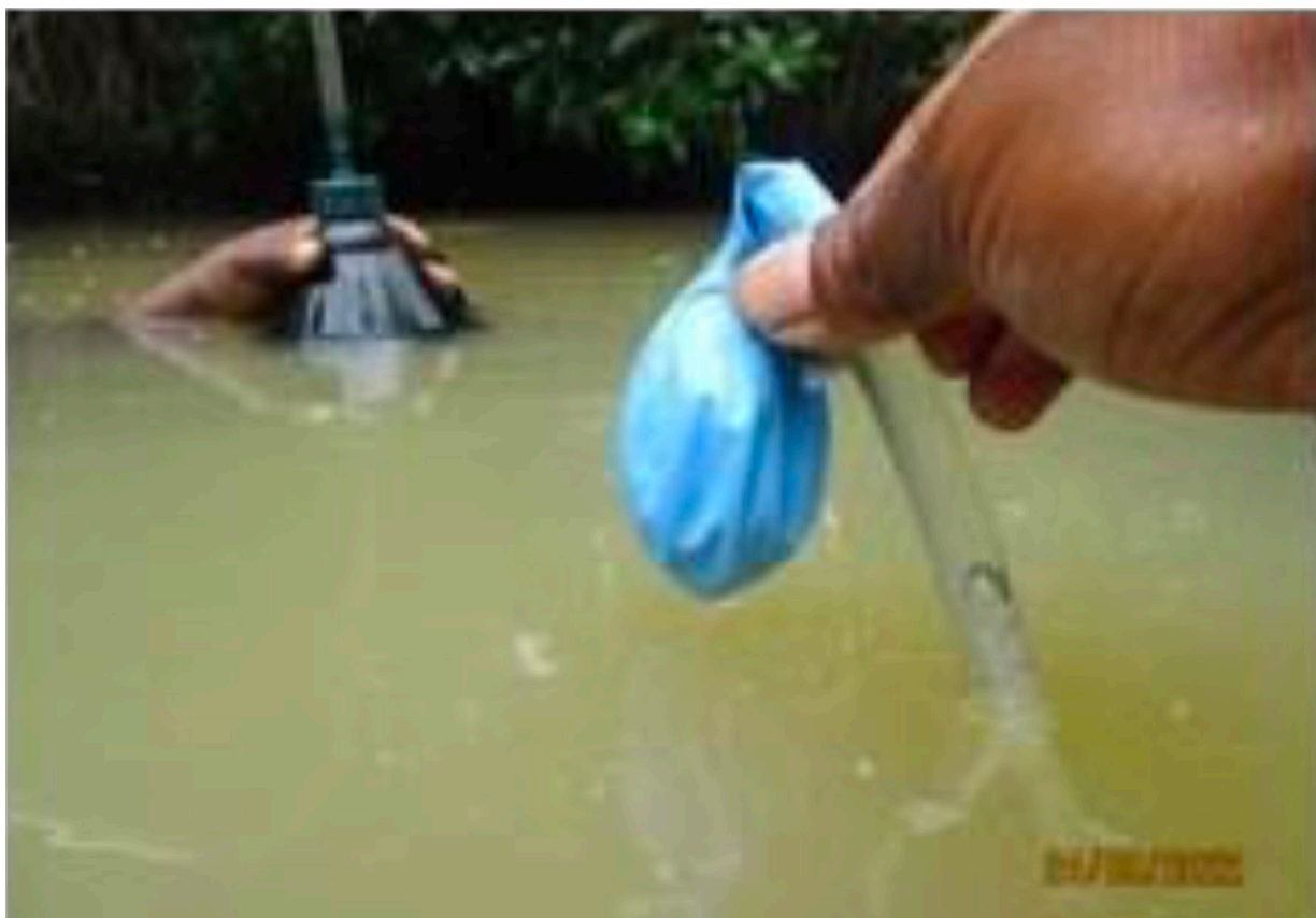
Figure 1. Collection of gas samples at Alligator Creek
