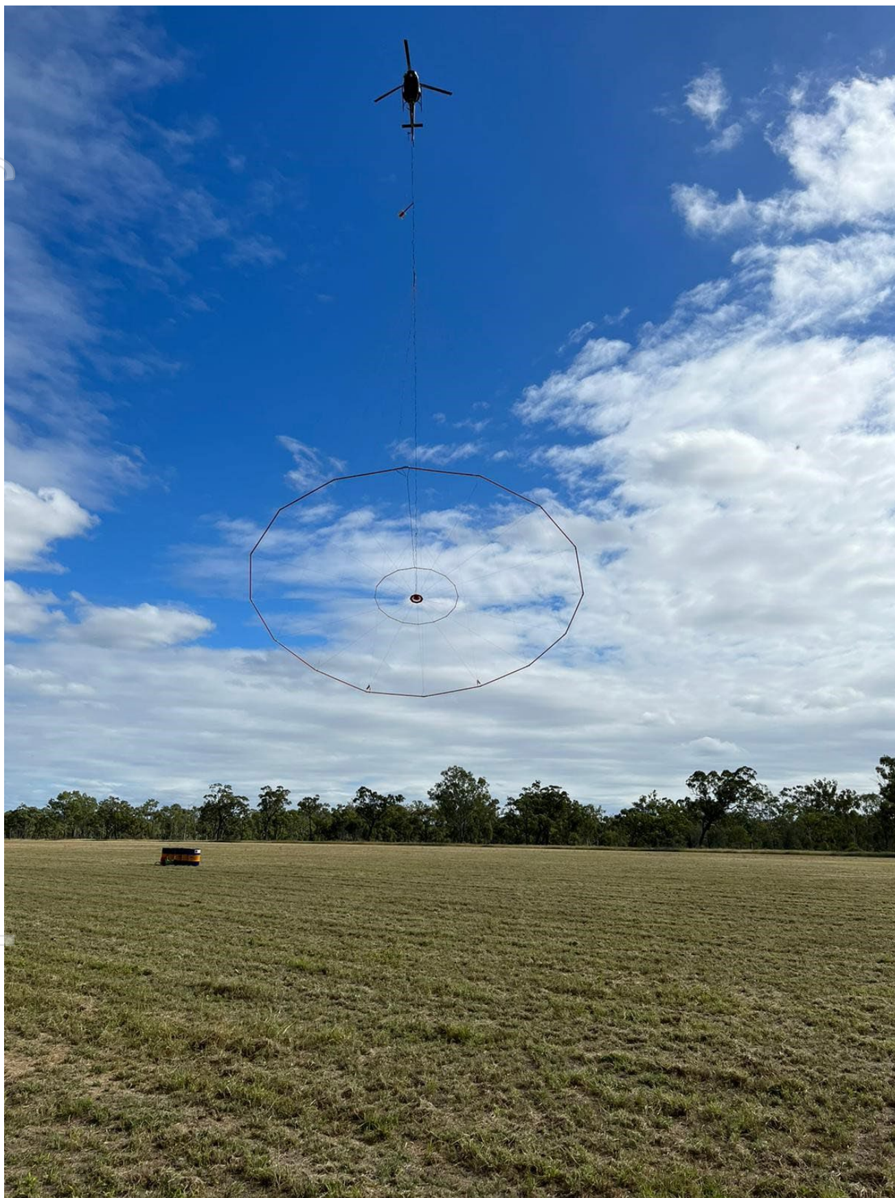
Figure 9. Airborne Heli-VTEM Survey underway at the Ravenswood North Project, June 2022.
