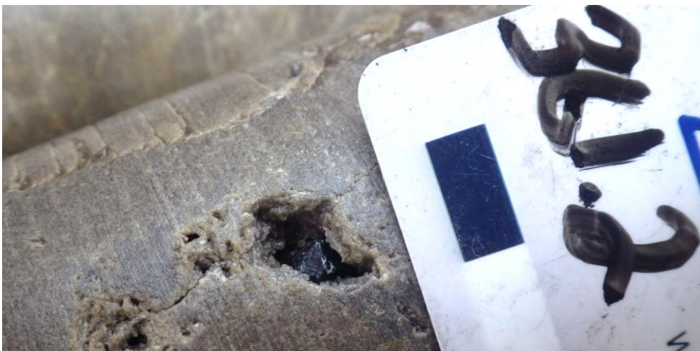
Figure 2: Sphalerite crystal sitting within a vug in drill hole ST22-10 (361.2m downhole).
