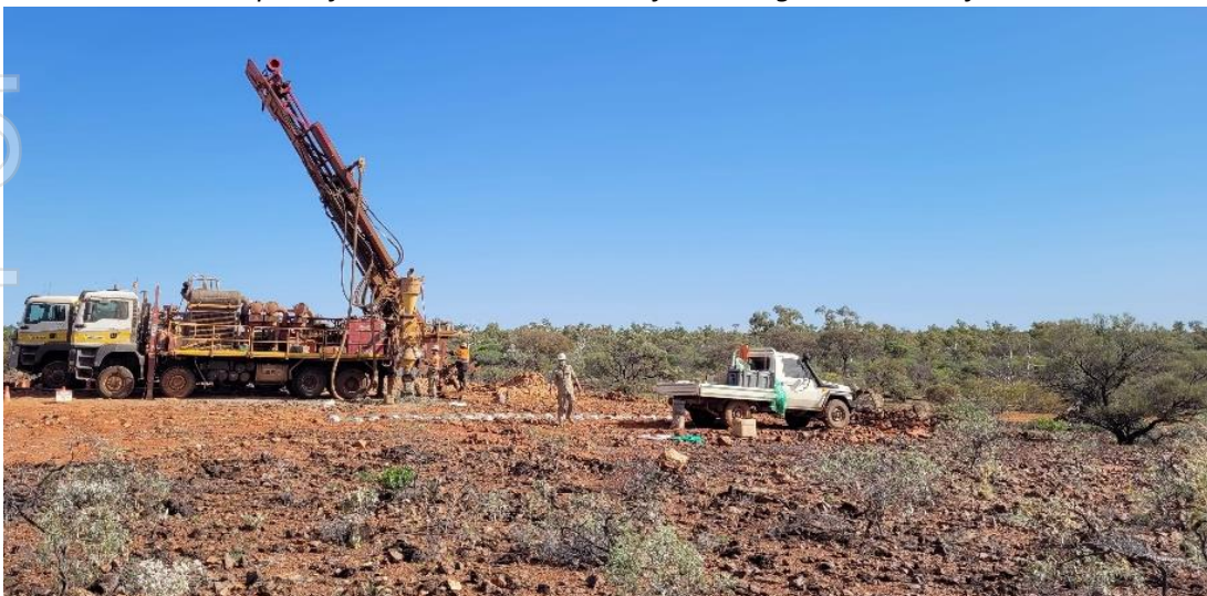
Figure 1: Photo of the RC drill rig commencing fence line drilling at the C3 carbonatite.
