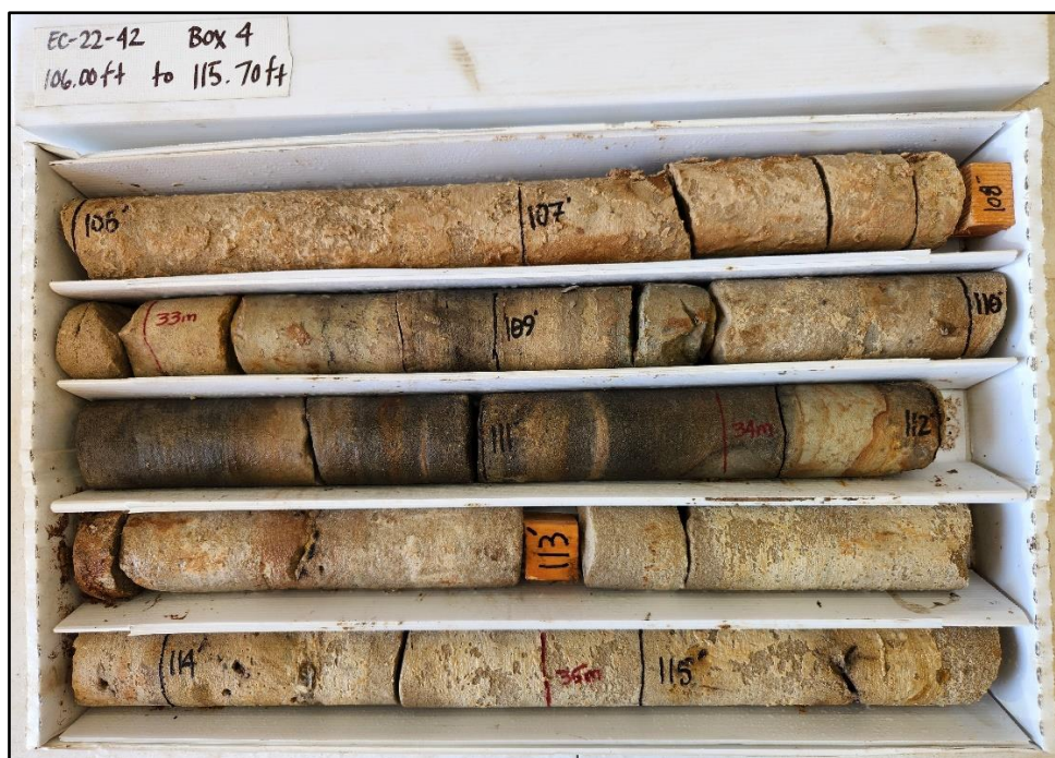
Figure 2: Drill hole ECDD42 core showing visible mineralisation and zone of elevated radioactivity (metre marks in red)
