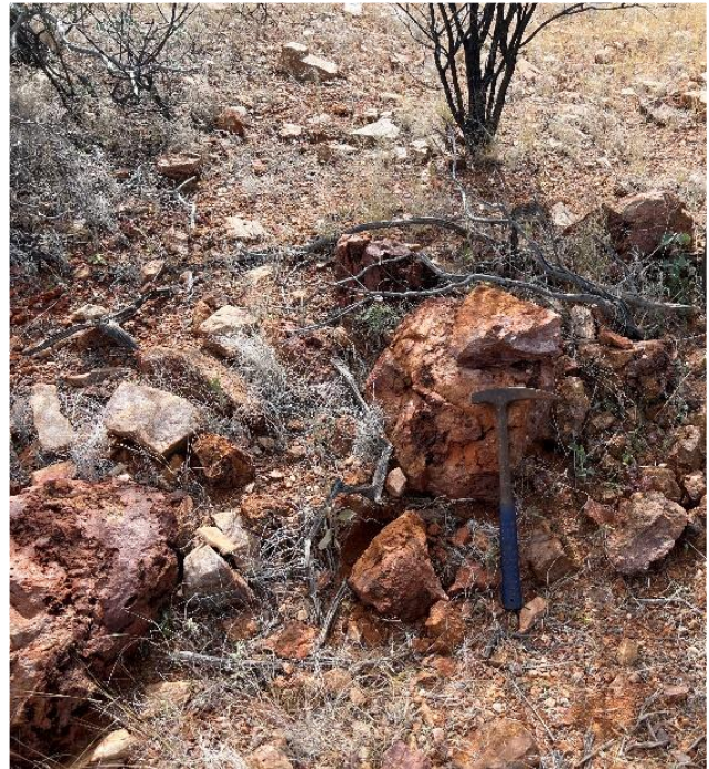
Figure 7: Monazite sample MWGS0708 which assayed 40.02% TREO with 6.40% \text{Nd}_2\text{O}_3 + \text{Pr}_6\text{O}_{11} .
