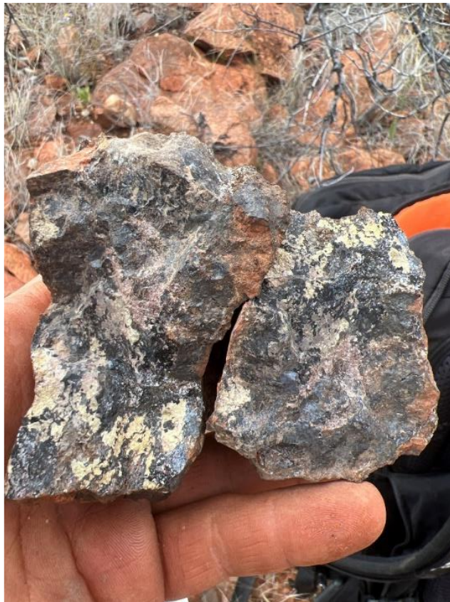
Figure 8: Monazite (pale red) rich carbonatite samples MWGS0769 (left) and MWGS0770 (right) which assayed 21.55% TREO with 3.74% Nd_2O_3 + Pr_6O_{11} and 15.19% TREO with 2.56% Nd_2O_3 + Pr_6O_{11} .
