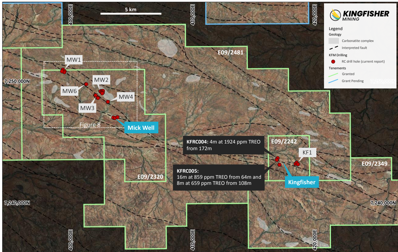
Figure 13: RC drilling results from the Kingfisher Prospect and the location of the Mick Well targets.
