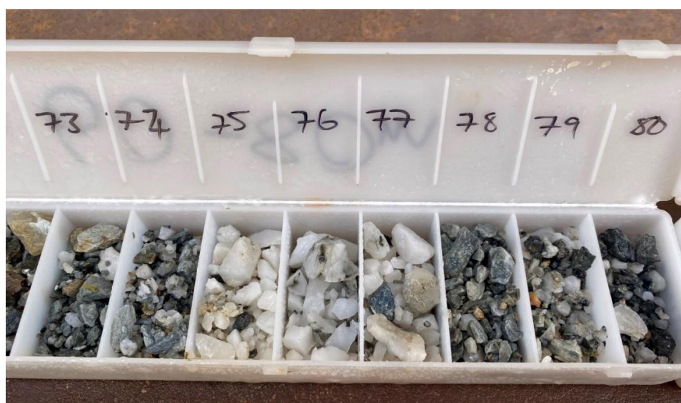
Figure 9. Photograph of RC drill chips from RD21008 (72 – 80 metres) showing quartz veining and sericite \pm chlorite alteration
