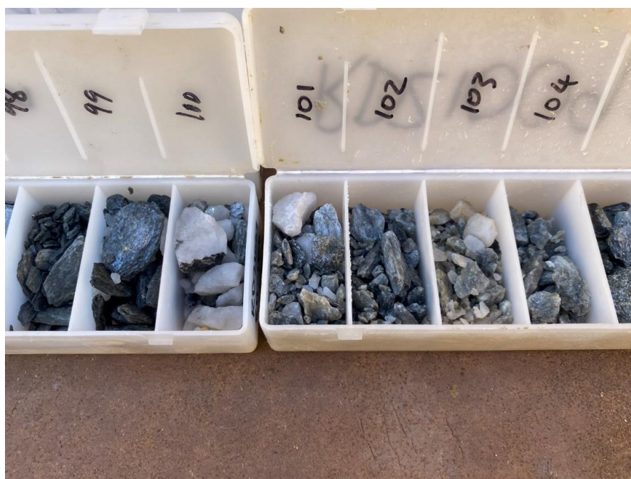
Figure 8. Photograph of RC drill chips from RD21009 (97 – 104 metres) showing visible sulphide and quartz veining present
