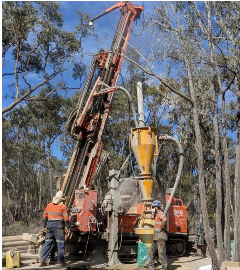
Figure 16: RC drilling at Fentiman's Reef prospect, South Muckleford Gold Project
