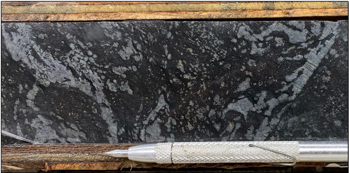
Figure 5: Recrystallised ultramafic rock with disseminated sulfide from 81 m zone assaying 0.21 % Ni from 65.36 m. Half NQ2 (51 mm) drill core.
