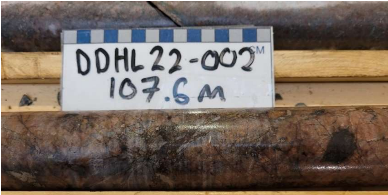
Figure 5: Trace uraninite mineralisation in DDHL22-002
