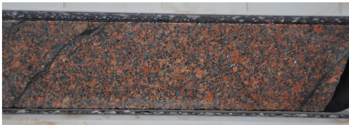
Figure 3: 22MEDD001 magnetite, hematite, albite, sericite, chlorite and epidote alteration in monzodiorite at 702m
