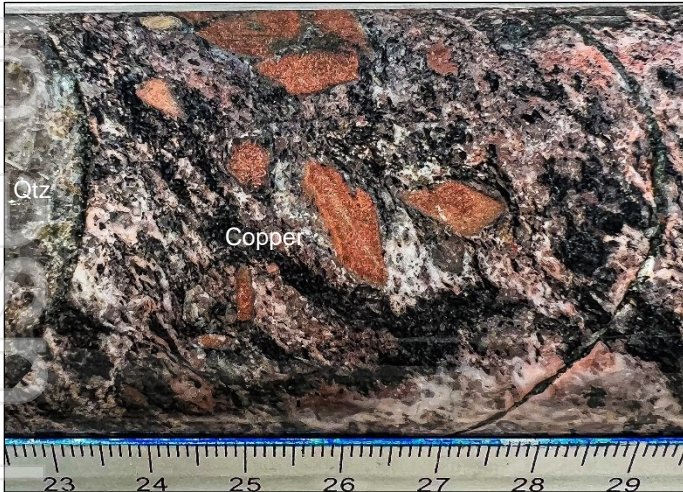
Figure 7a Breccia with native copper replacing basalt clasts. Quartz vein to the left contains crystalline native copper. Strong biotite (black), silica (clear) and hematite dust (pink) alteration.
