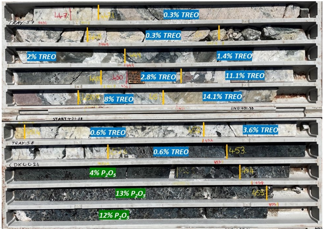
Figure 2. CDX0020 447-456m: rare earths and phosphate mineralised intersection of 11.6m at 1.9% TREO and 7% P 2 O 5 including 1.2m at 11.4% TREO and 8% P 2 O 5 .
