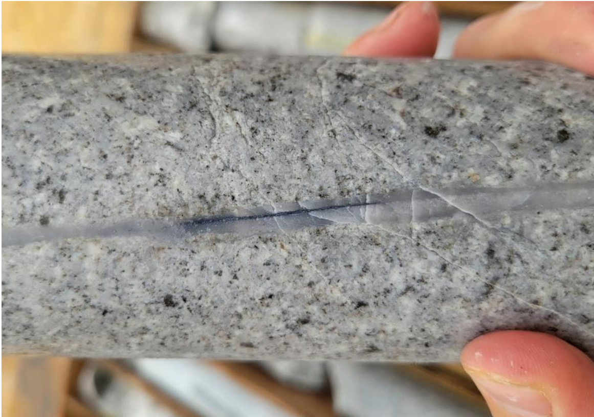
Figure 5: Molybdenite within quartz vein in drill core from WD22-01C at approximately 744.29m (2442ft).
