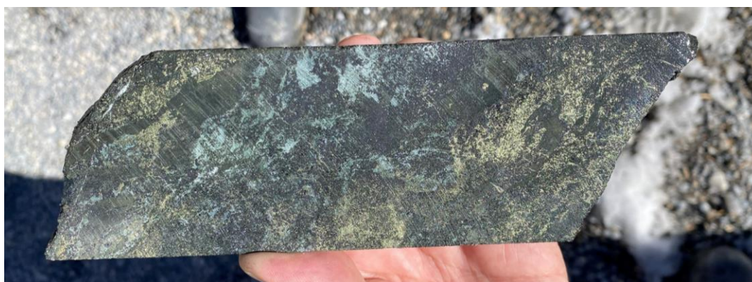
Figure 1: Chalcopyrite rich magnetite skarn in drill core from 422m (1,385ft) downhole in WD22-01C
