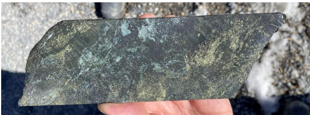
Figure 1: Chalcopyrite rich magnetite skarn in drill core from 422m (1,385ft) dowhole in WD22-01C
