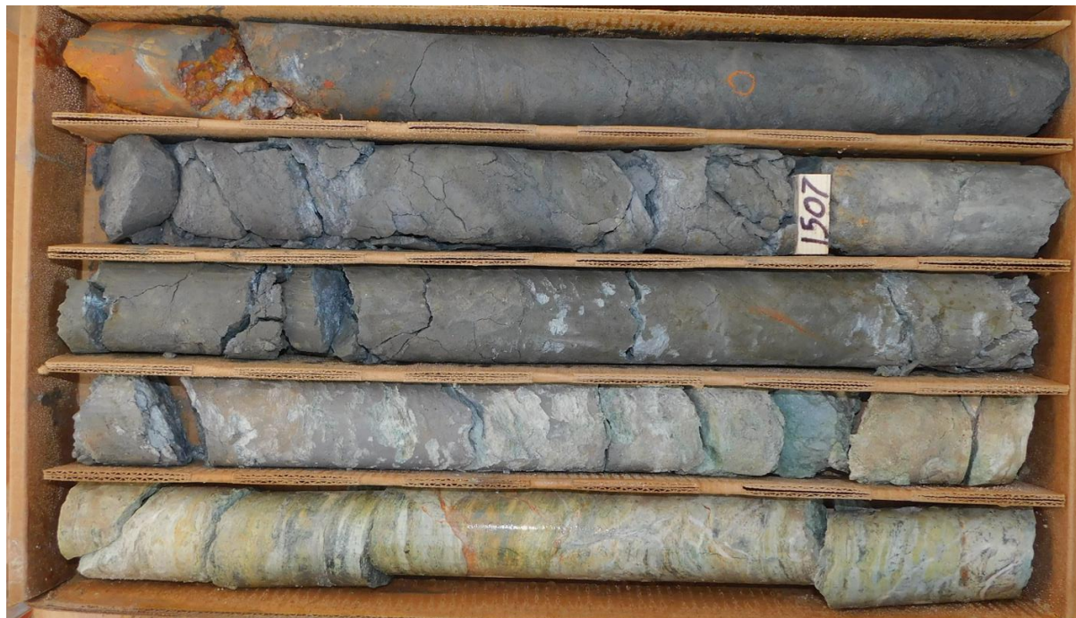
Figure 2: Photo of massive zinc sulphide in WD22-19 between 457.6 – 460.3m (1501.5 – 1510.5ft) downhole.
