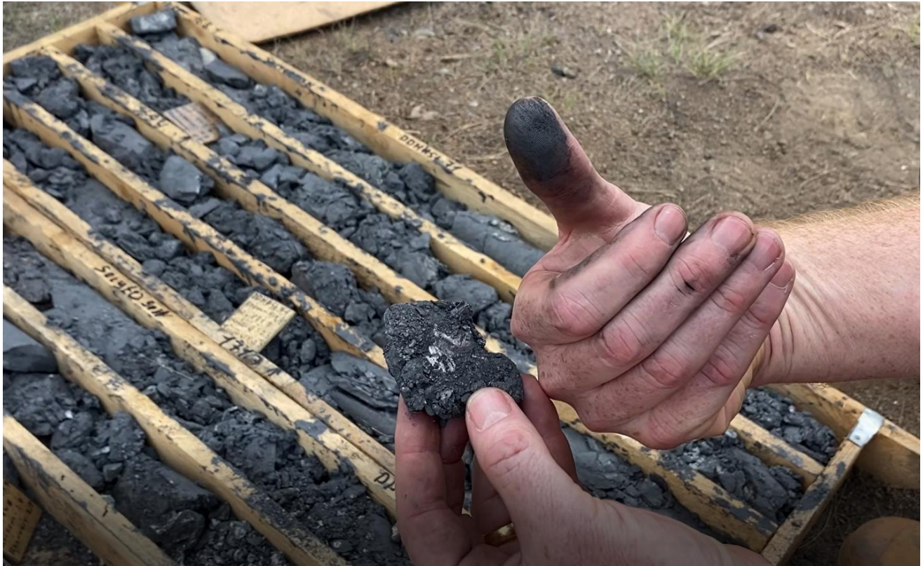
Figure 1 - High-grade graphite at 170m in ST-71 to the north-east of the CGZ
