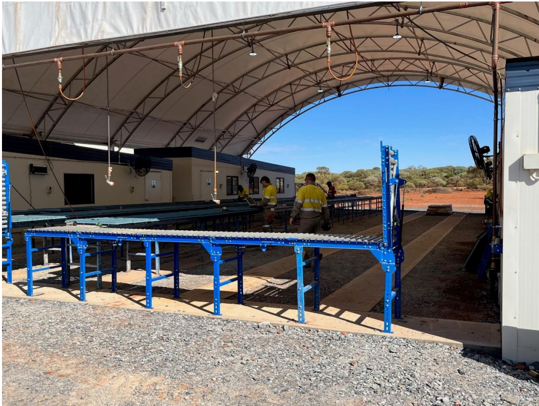
Figure 14 – Underground grade-control diamond core processing.
