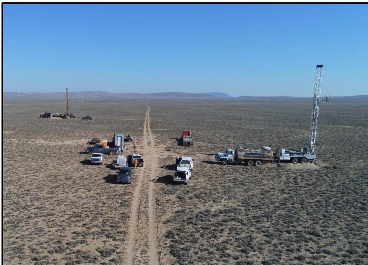
FIGURE 1. MUD ROTARY DRILL RIGS OPERATIONING, THOR ISR URANIUM PROSPECT, GDB WYOMING.
