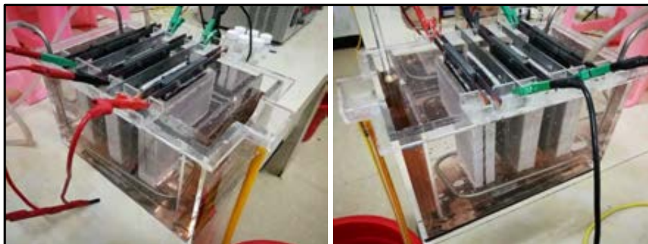
Figure 13-25: One of Electrowinning Test Devices
