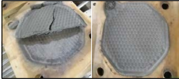
Figure 13-29: Filtration Cakes – Non-Magnetic Tailings (12.6% w/w Moisture)
