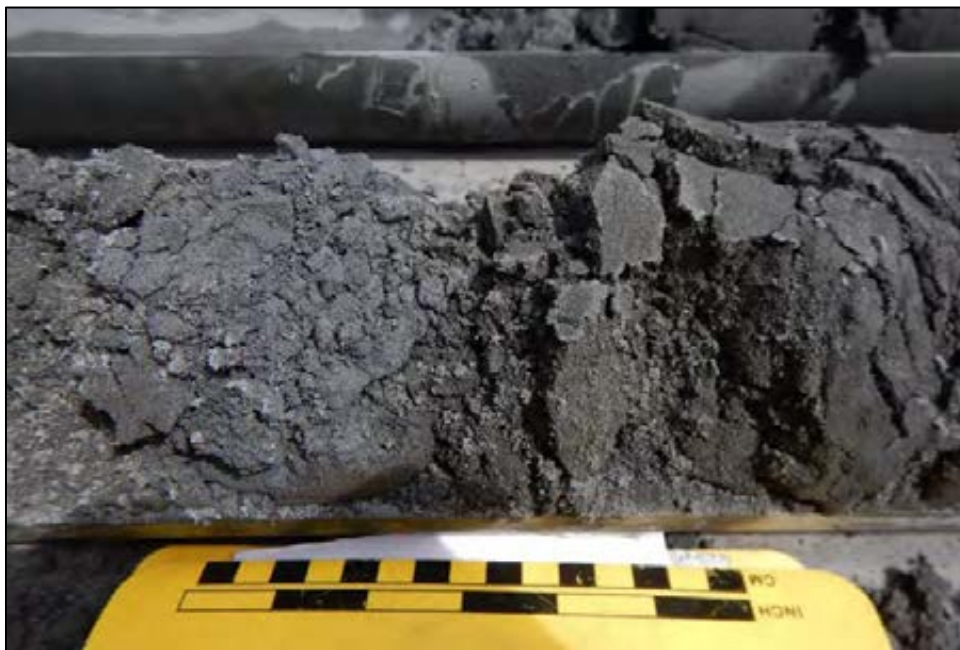
Figure 12-3: Close-up of Tailings Material, T2P-346, Sample TT18-001
