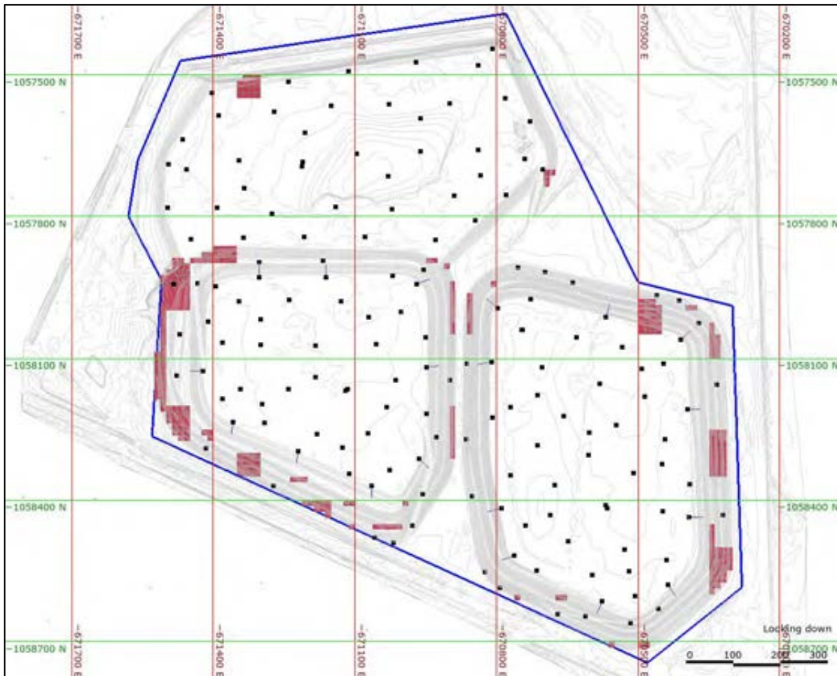
Figure 14-13: Plan View Showing Extent of Indicated Resource Blocks (Red); Measured Blocks are not Shown (All Remaining Blocks)
