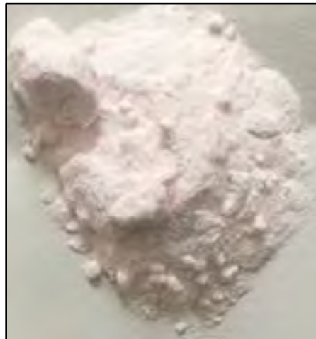
Figure 13-37: HPMSM Produced from the Selenium- and Chromium-free 99.9% HPEMM Flakes
