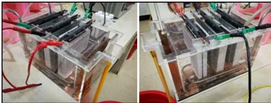
Figure 13-25: One of Electrowinning Test Devices
