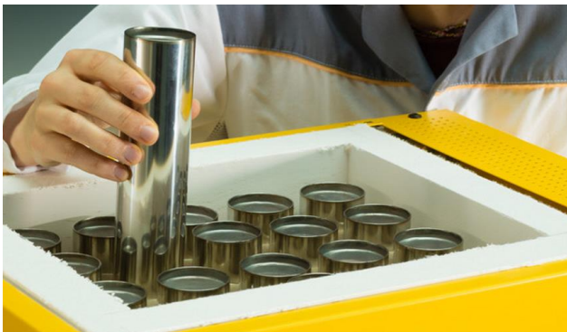
Figure 1 – SAS cells in battery module
