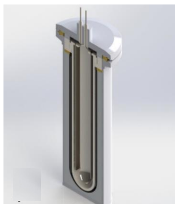
Figure 6 – Cross section of CERENERGY® Battery
