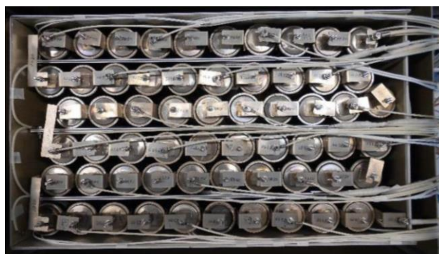
Figure 8 – Configuration of cells in battery module
