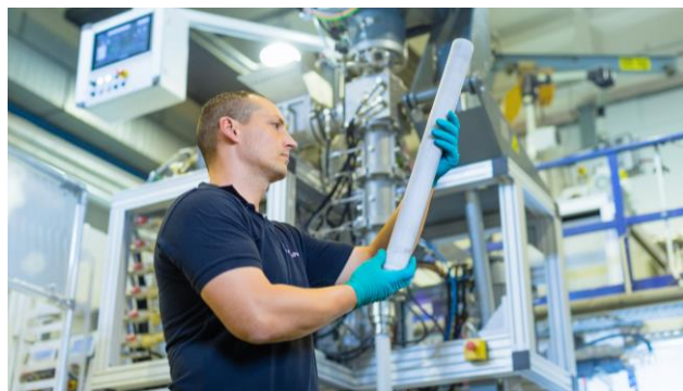
Figure 3 – Ceramic solid-state electrolyte at IKTS pilot facility
