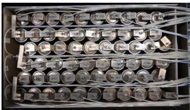
Figure 8 – Configuration of cells in battery module
