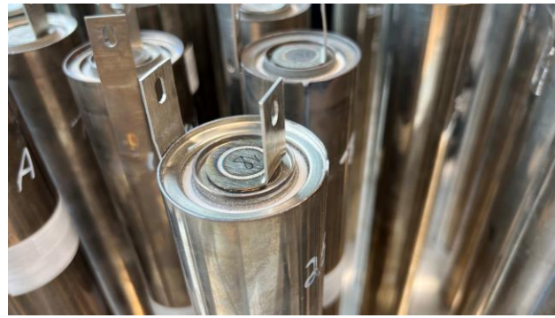
Figure 4 – SAS cell with positive and negative terminal
