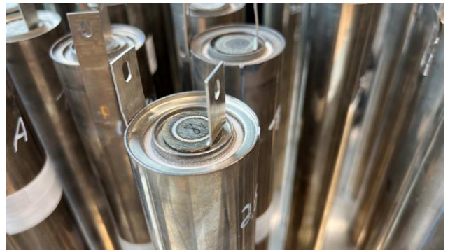
Figure 4 – SAS cell with positive and negative terminal
