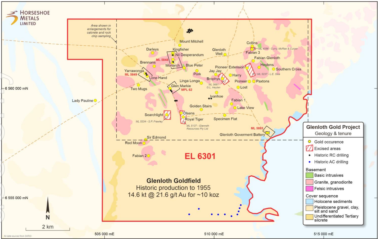
Figure 15: Location of Glenloth Goldfield tenure with regional geology and named gold occurrences
