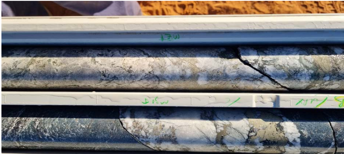
Figure 8-1: Drill core used for metallurgical studies
