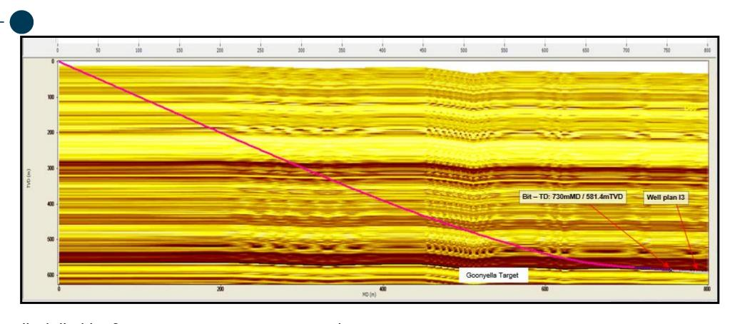
Lateral wells drilled by Sperry using gamma imaging tool.
