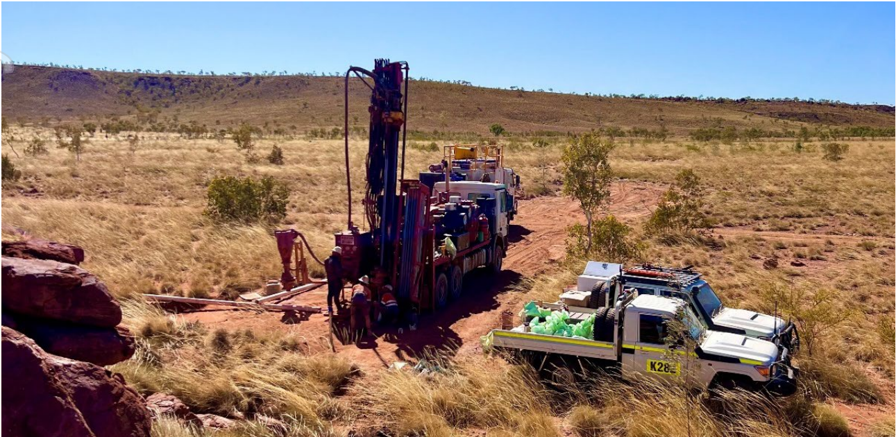
Figure 1: RC drilling at the Tanami Heavy REE Project, WA.
