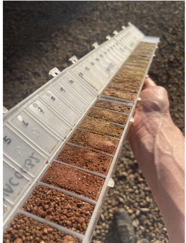
Figure 4 and 5: Kasiya drilling sample collection under the cyclone and mineralised weathering profile displayed in a chip tray
