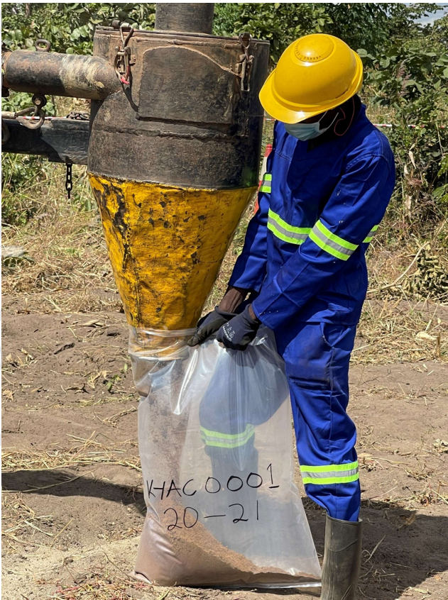
Figure 4 and 5: Kasiya drilling sample collection under the cyclone and mineralised weathering profile displayed in a chip tray
