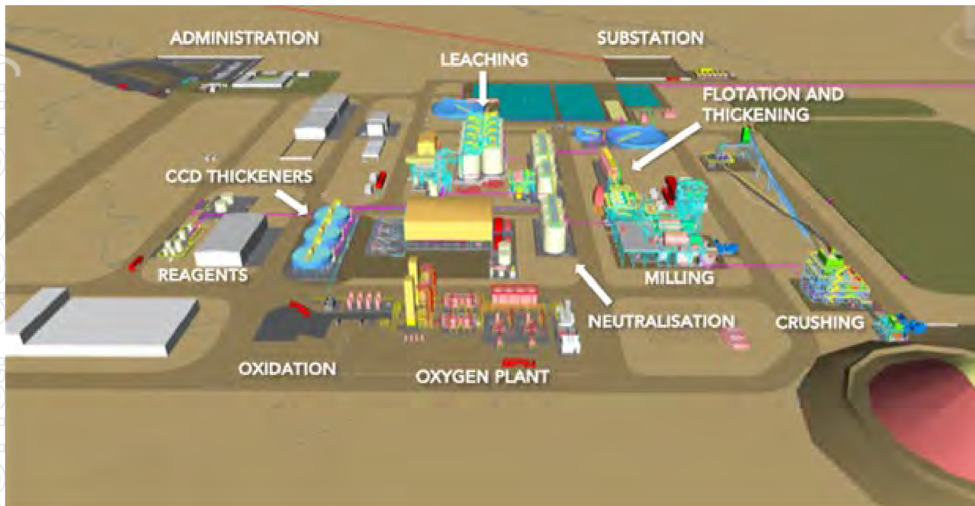
Figure 13: Plant Layout from crusher stockpile
