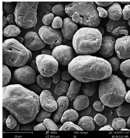
SEM micrograph of Maniry spheronised & purified product; magnification 3,000x
