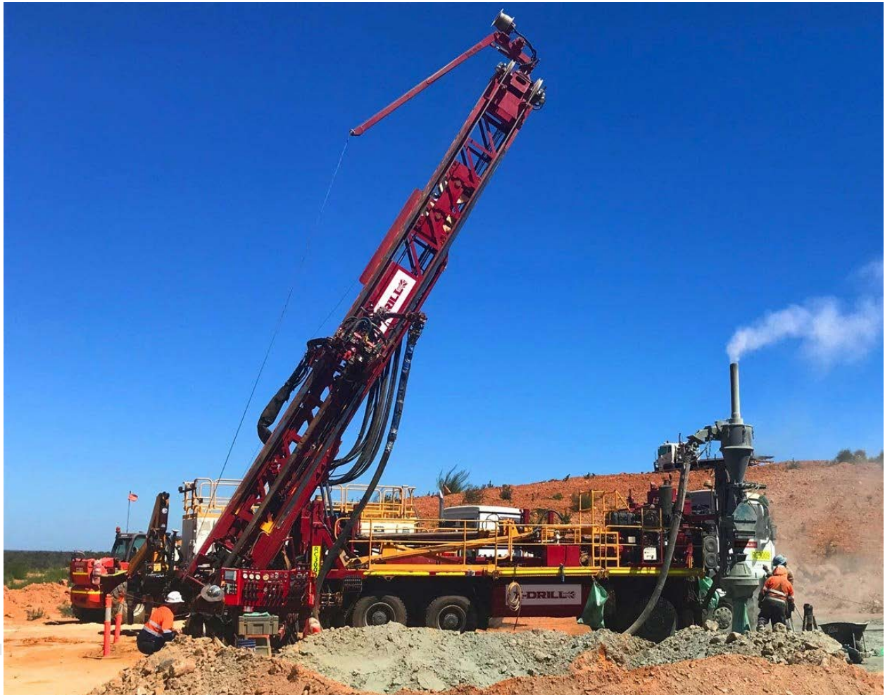
Figure 1. Showing the K-Drill RC rig that will perform the infill drilling at the Manna Lithium Project
