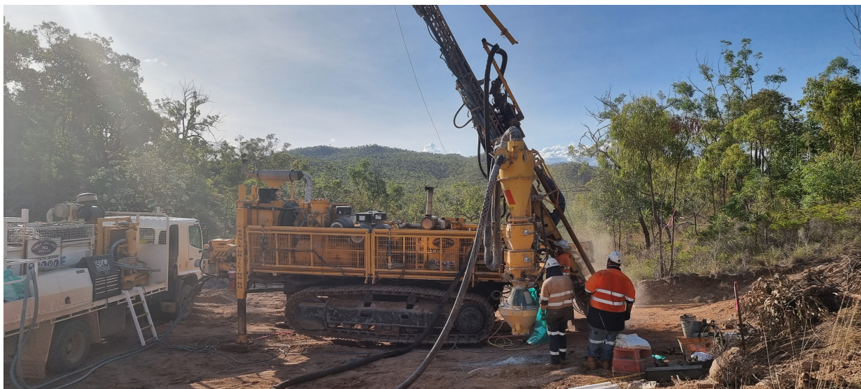
Figure 1 – RC drilling at Adelaide Prospect
