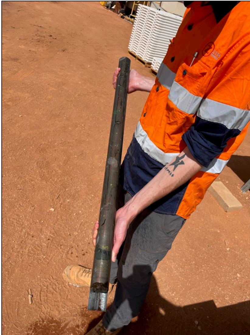
Figure 1: Diamond drill core of massive Ni-sulphide intersected in TED42, the follow-up hole to the Dimma discovery hole, TED41. See text for further details.
