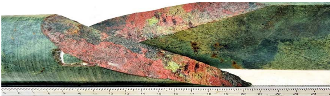
Figure 4 LEFD006 interval 224.5 to 224.8m shows high-magnesium Western Basalt, mineralised by native copper along fracture plane with a gypsum film, with epidote alteration and minor ex-sulphides (LEX ASX release 1 August 2022)
