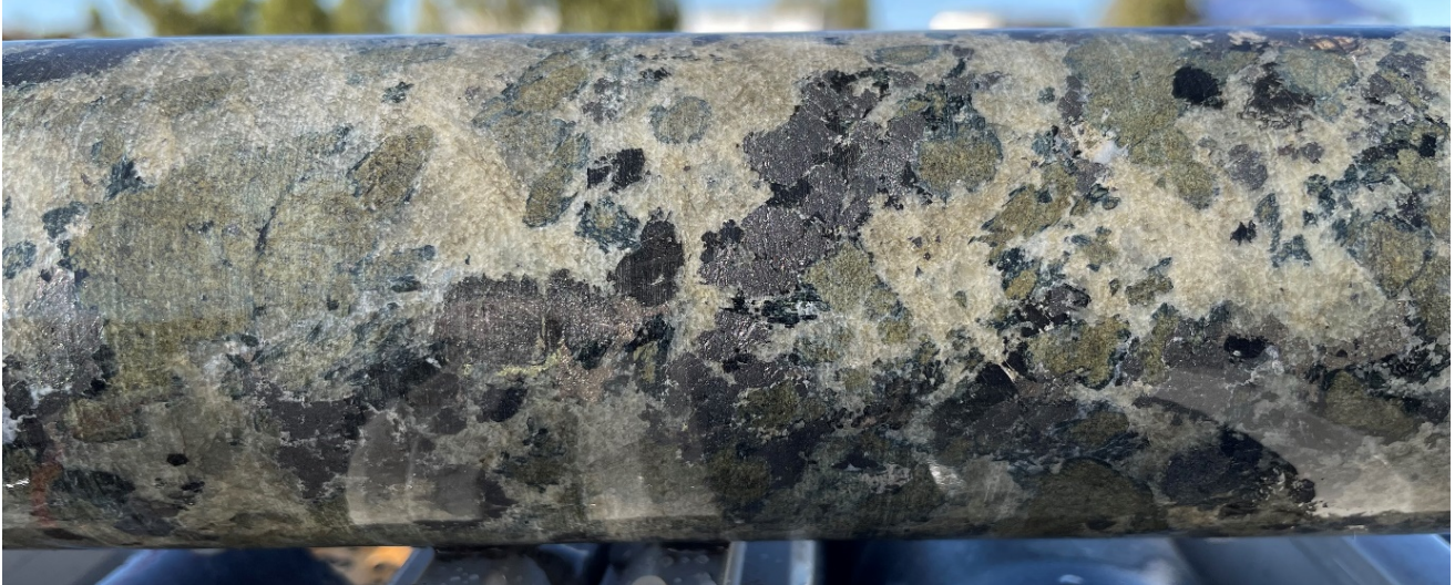
Figure 1. Example of Phoscorite in core, Apatite= light brown, Diopside=green, Magnetite=dark grey, Phlogopite=black
