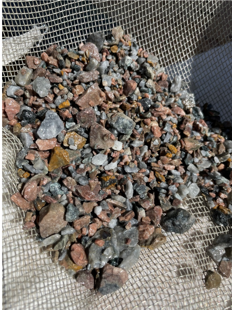
Figure 3. Strong (>5% monazite and bastnasite) mineralisation in Carbonatite dyke from 99-100m in hole CDX0084. Monazite=brown, Bastnasite=pink, Carbonatite=grey-white
