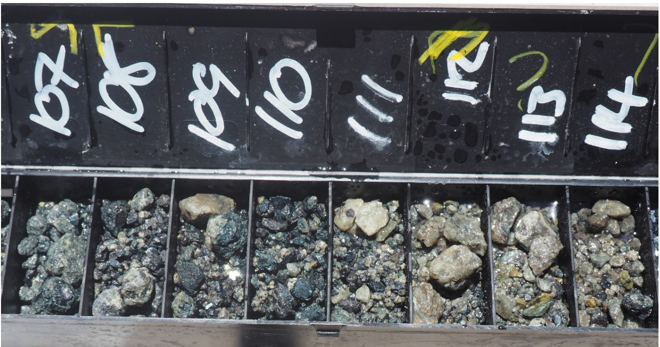
Figure 2. Strong Apatite (light brown) mineralisation (>15% apatite) in phoscorite. Hole CDX0093 at 107m – 114m
