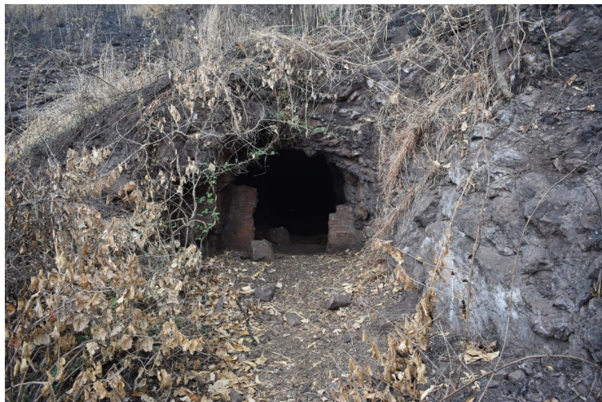
Above: Old underground adit into the north zone of dolomite carbonatite mineralisation. The adit is about 1.5m x 1.5m and extends for about 300m into the hill toward the south.
