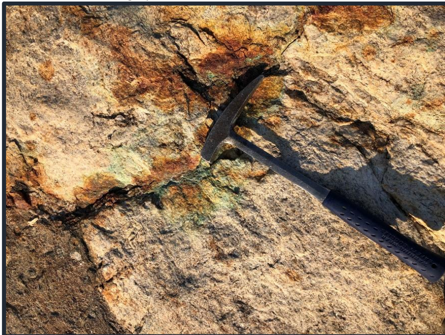
Figure 2: A mineralised ferruginous Quartz vein containing gold, copper and pyrite crosscutting a calc-silicate and granitic dike
