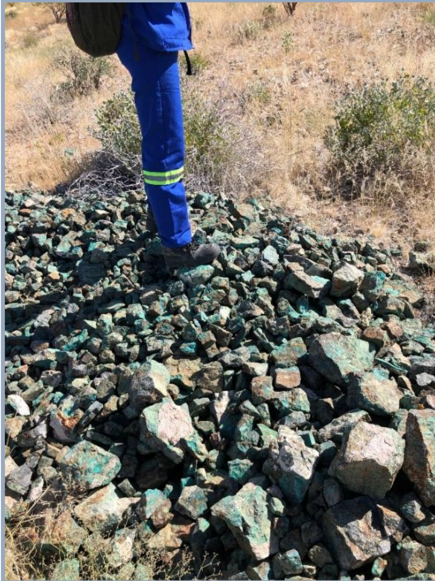
Figure 7: Example 2 of historical workings on the copper rich zones (oxides; chrysocolla, malachite and subordinate azurite whereas sulphides are chalcopyrite, bornite and chalcocite) hosted within the calc-silicates
