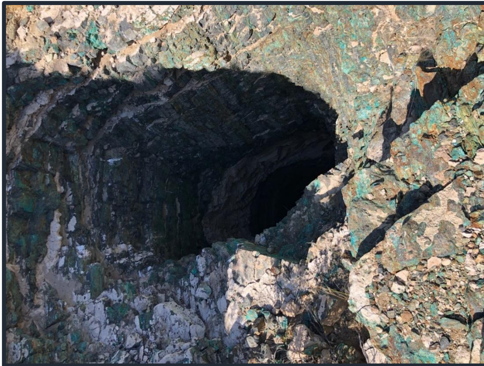
Figure 6: Example 1 of historical workings on the copper rich zones (oxides; chrysocolla, malachite and subordinate azurite whereas sulphides are chalcopyrite, bornite and chalcocite) hosted within the calc-silicates
