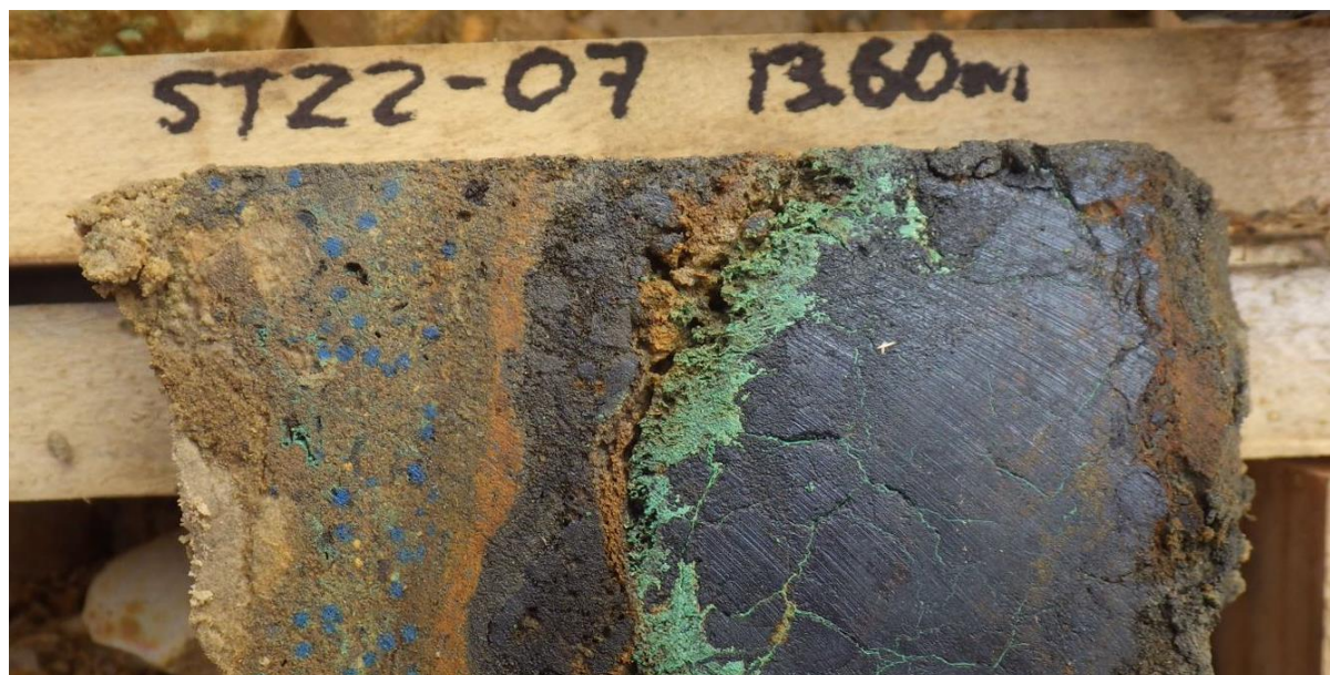
Figure 4: Drill core from ST22-07 from 13.6m downhole showing a mix of copper oxides developed on the outside edge of a massive chalcocite band (azurite – blue, malachite – green/aqua, chalcocite – dark grey).
