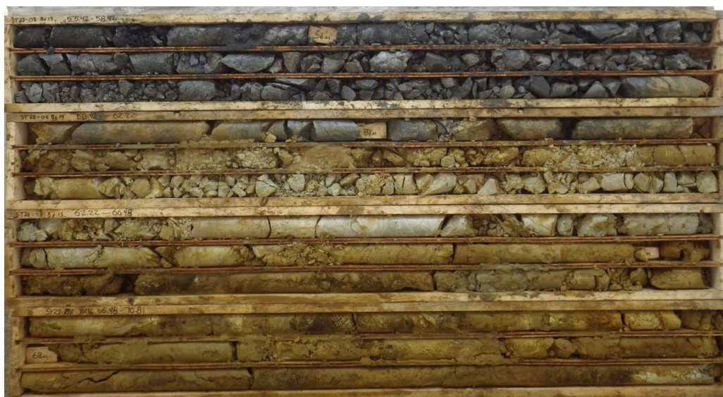
Figure 5: Drill core from ST22-08 between 55.42 – 70.81m downhole – note strong chalcocite (dark grey) in upper core box
