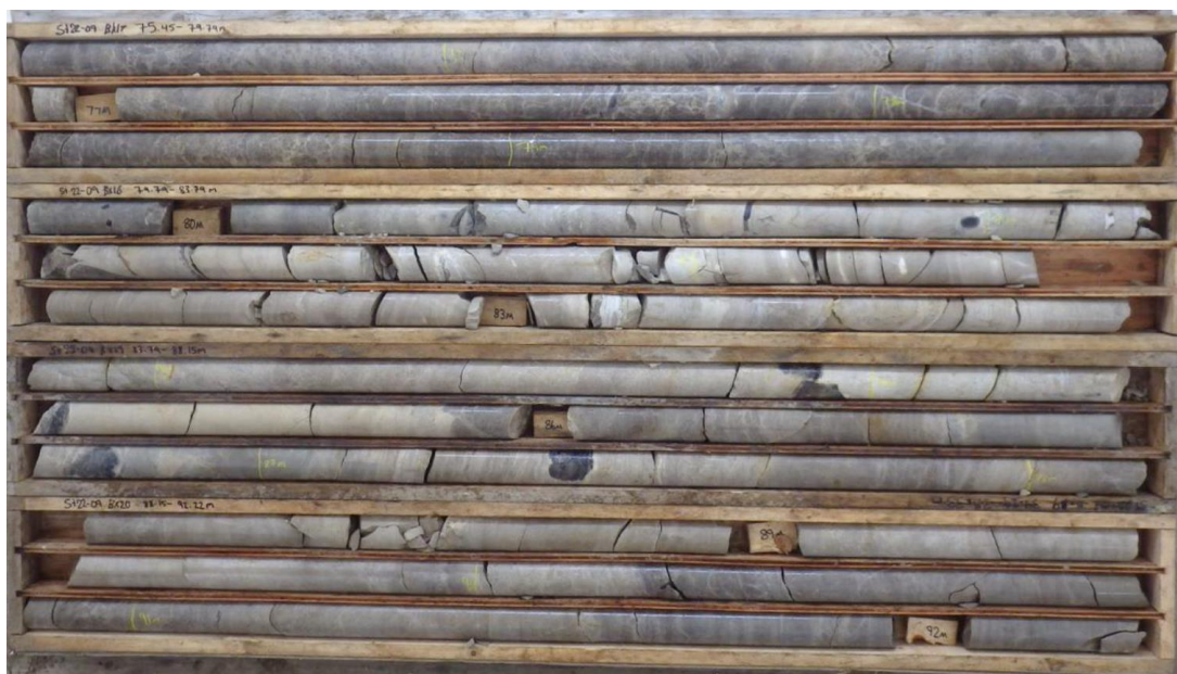
Figure 6: Drill core from ST22-09 between 75.45– 92.22m downhole showing dark gray chalcocite veining
