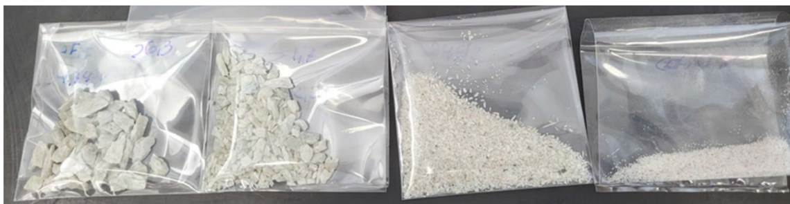
Figure 1: Spodumene concentrate samples from 3.0g/cm 3 HLS across the four tested size fractions
