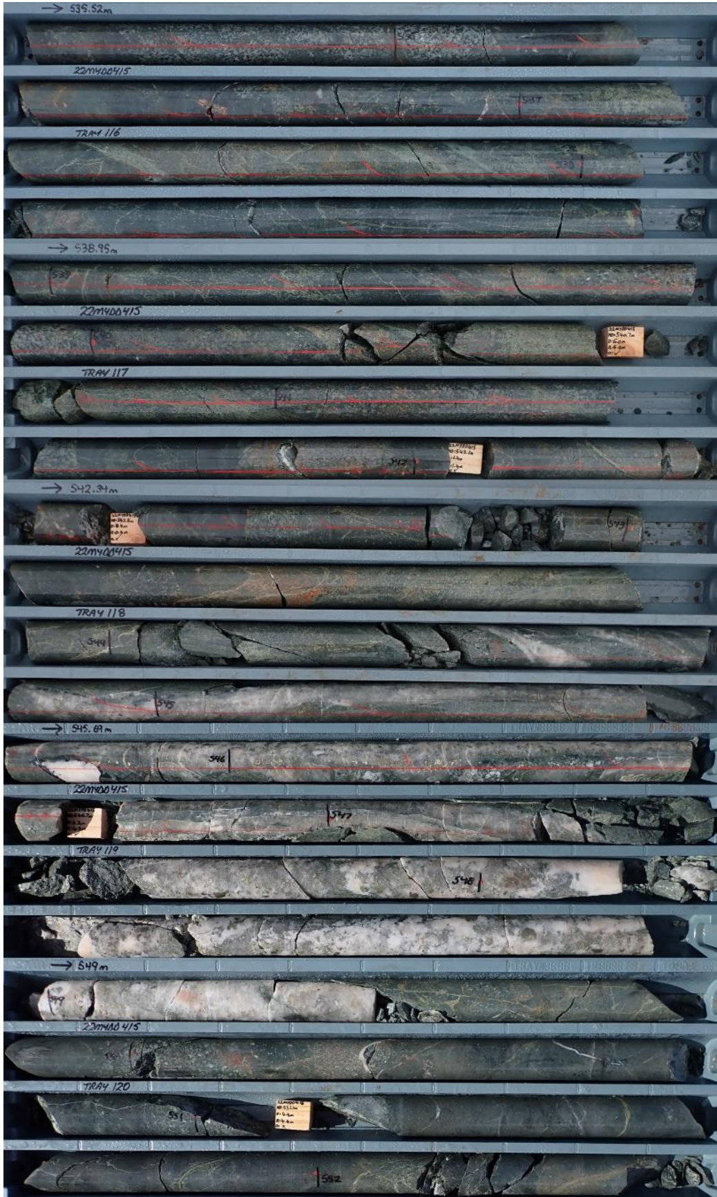
Figure 7. Drill core from hole 22MYDD415 between 535.5 and 552.4m highlighting the highly altered nature of the variably mineralised interval. Note the intense quartz-carbonate-chalcopyrite-pyrite veining (white) in this interval. Close-up images highlighting specific rock types, alteration styles and sulphide mineralisation are shown in Figures 3-6 .
