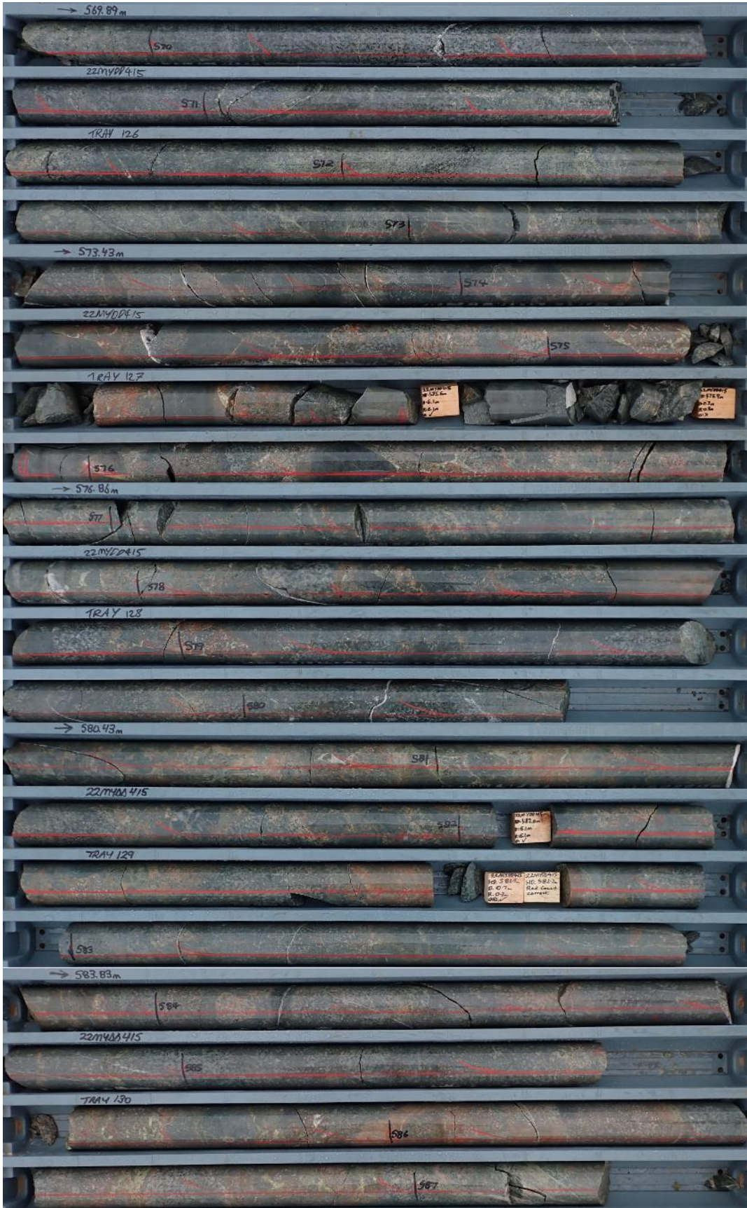
Figure 9. Drill core from hole 22MYDD415 between 569.9 and 587.2m highlighting the highly altered and polymict nature of the variably mineralised interval. Close-up images highlighting specific rock types, alteration styles and sulphide mineralisation are shown in Figures 3-6 .
