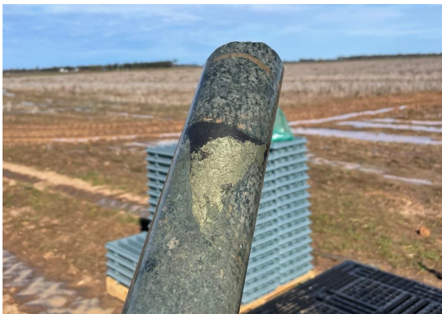
Figure 6. Section of strongly altered diorite with a very large patch (to ~80mm) of chalcopyrite (yellow) and magnetite (black) from 714 metres down hole in 22MYDD415.
