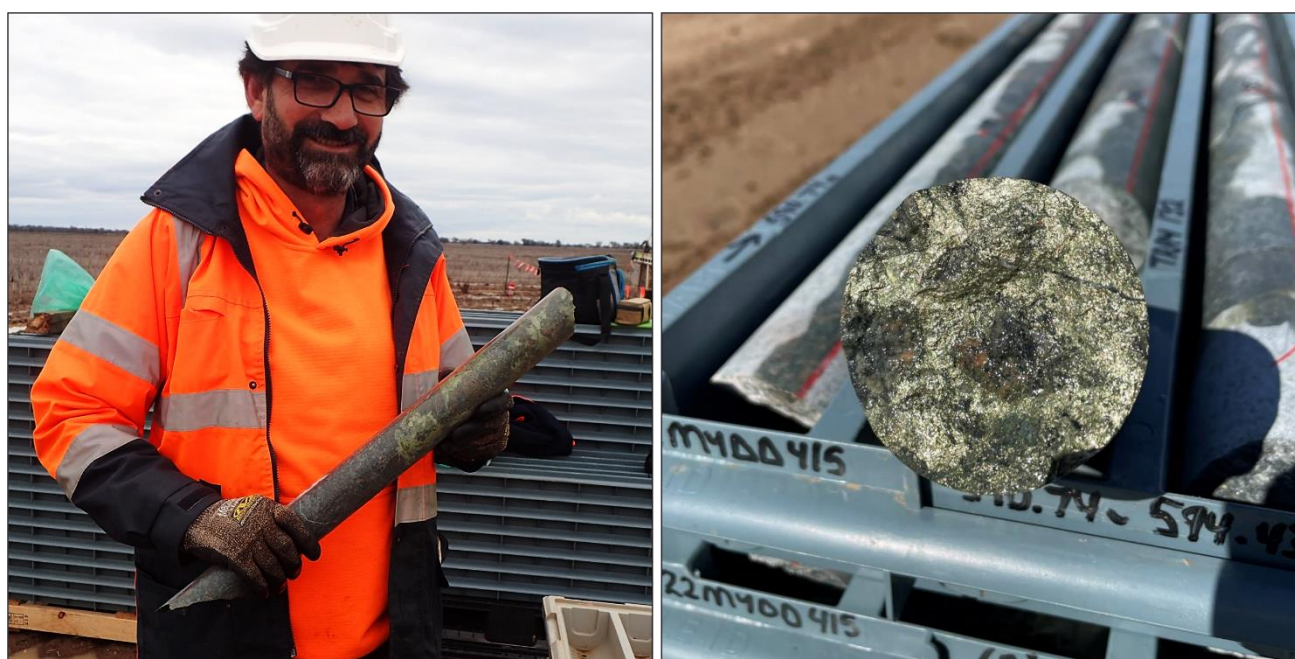
Figure 3. Magmatic Resources' Exploration Manager, Steven Oxenburgh, holding core with abundant breccia-hosted chalcopyrite (yellow) from 588m down hole (left); and cross section of core from 591.6m down hole displaying semi-massive, breccia hosted chalcopyrite (right).
