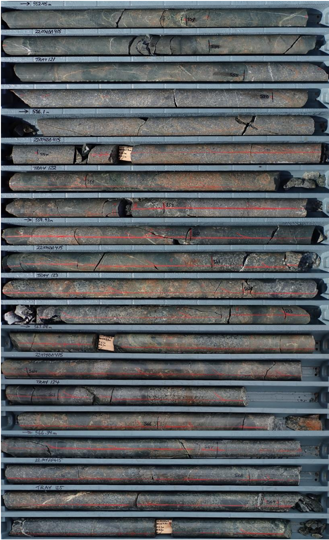
Figure 8. Drill core from hole 22MYDD415 between 552.4 and 569.9m highlighting the highly altered and polymict nature of the variably mineralised interval. Close-up images highlighting specific rock types, alteration styles and sulphide mineralisation are shown in Figures 3-6 .
