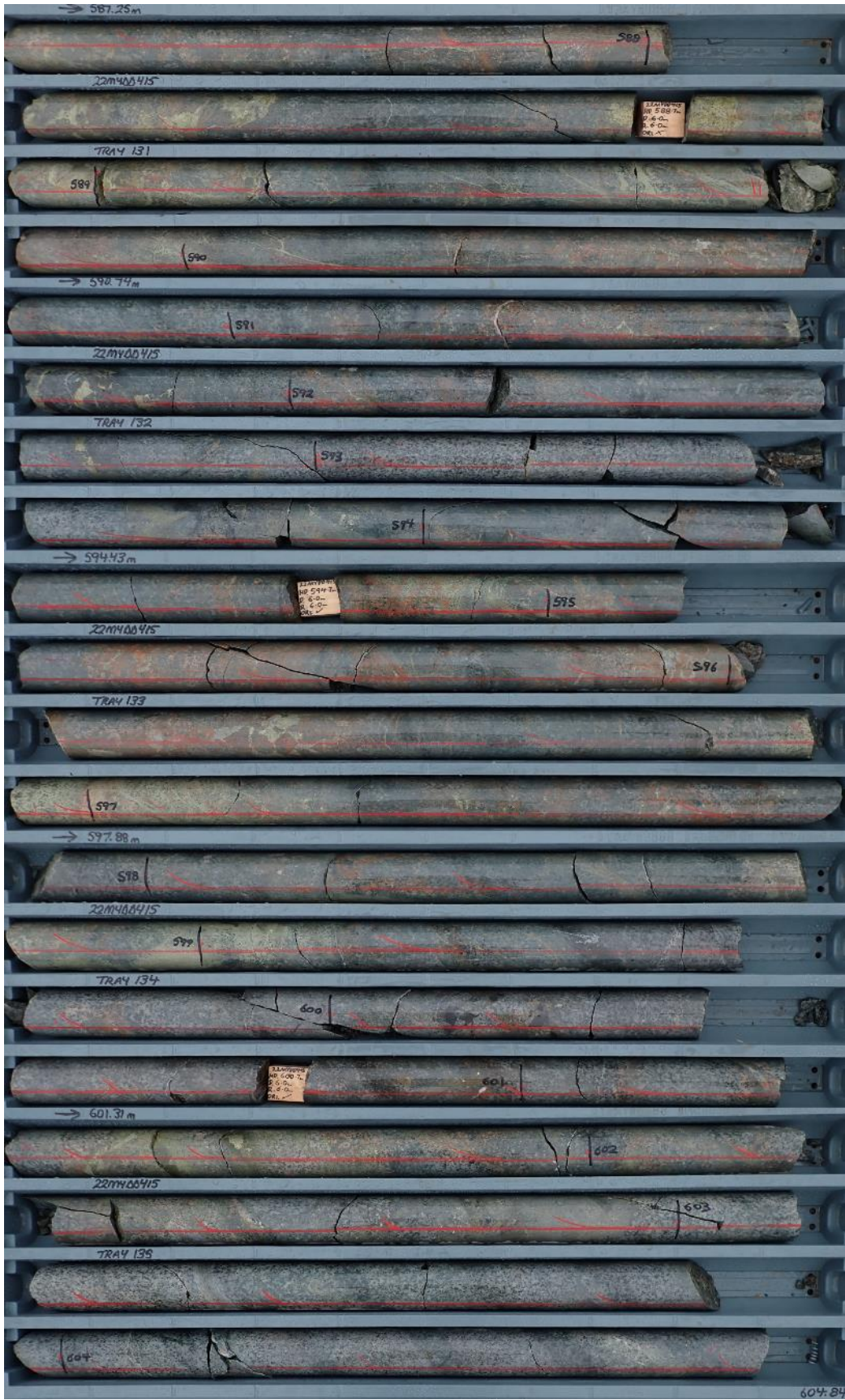
Figure 10. Drill core from hole 22MYDD415 between 587.2 and 604.8m highlighting the highly altered and brecciated zone with strong chalcopyrite/epidote development (yellow). Close-up images highlighting specific rock types, alteration styles and sulphide mineralisation are shown in Figures 3-6 .
