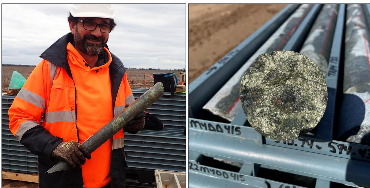
Figure 3. Magmatic Resources' Exploration Manager, Steven Oxenburgh, holding core with abundant breccia-hosted chalcopyrite (yellow) from 588m down hole (left); and cross section of core from 591.6m down hole displaying semi-massive, breccia hosted chalcopyrite (right).
