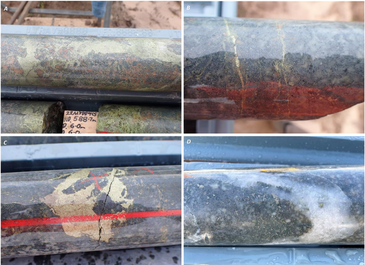
Figure 5. Images of various down hole intervals of HQ drill core (63.5mm diameter) from the lower portions of hole 22MYDD415. A) intense development of chalcopyrite (yellow) and epidote (green-yellow) within a K feldspar altered polymict breccia from ~588m; B) thin chalcopyrite-pyrite veins cross-cutting a pervasively chlorite-altered diorite from 595.2m; C) brecciated, chlorite-altered diorite strongly infilled with chalcopyrite and lesser pyrrhotite (brass-coloured, right) from 730.5m; D) chlorite-altered diorite with abundant disseminated pyrite, cut by quartz-carbonate veins with minor chalcopyrite from 810.2m.
