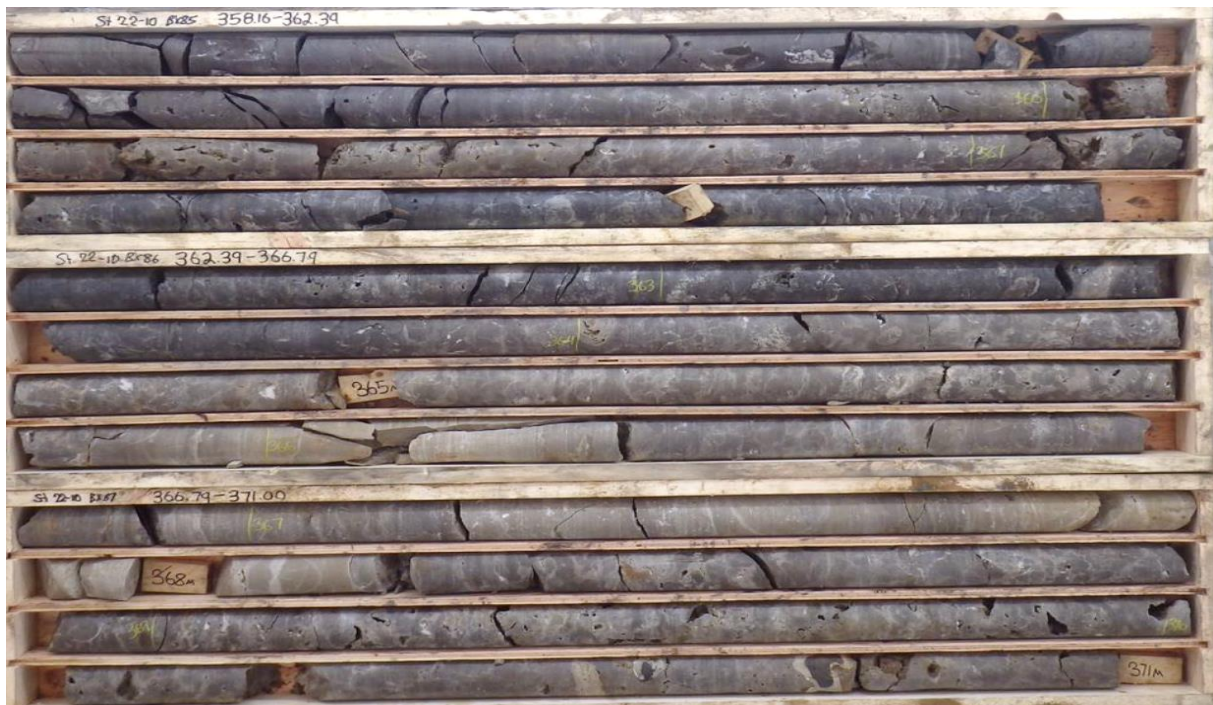
Figure 6: ST22-10 drill core between 358.16 – 371m downhole showing the vuggy nature of the carbonate rocks. The vugs can contain variable amounts of chalcopyrite, sphalerite, calcite, pyrite and bitumen.
