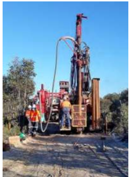
Figure 75 Air-core drilling rig
