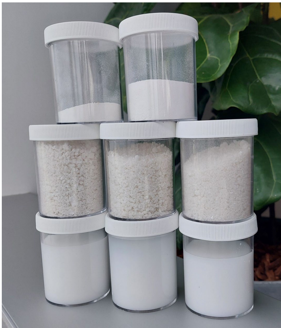
Figure 1: Samples from the micro-plant taken at different stages of the process, with final HPA top right
